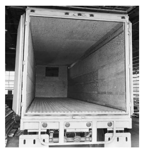
Sanded plywood is particularly well suited for materials handling applications where damage to the commodity or material being shipped or stored can be minimized by a smooth surface. For example, bins designed to handle soft fruits or vegetables are commonly made of sanded plywood. Similarly, smooth sanded plywood pallet decks can reduce damage to goods that might otherwise be torn or snagged by more abrasive or splinter-prone pallet decks.
